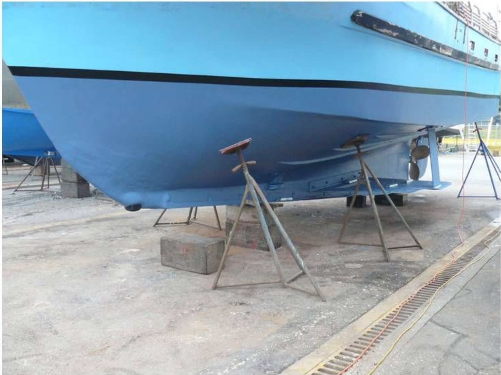
The Moody Blue has a draft of 6 feet and is equipped with batwing stabilizers and a forward-scanning sonar.
