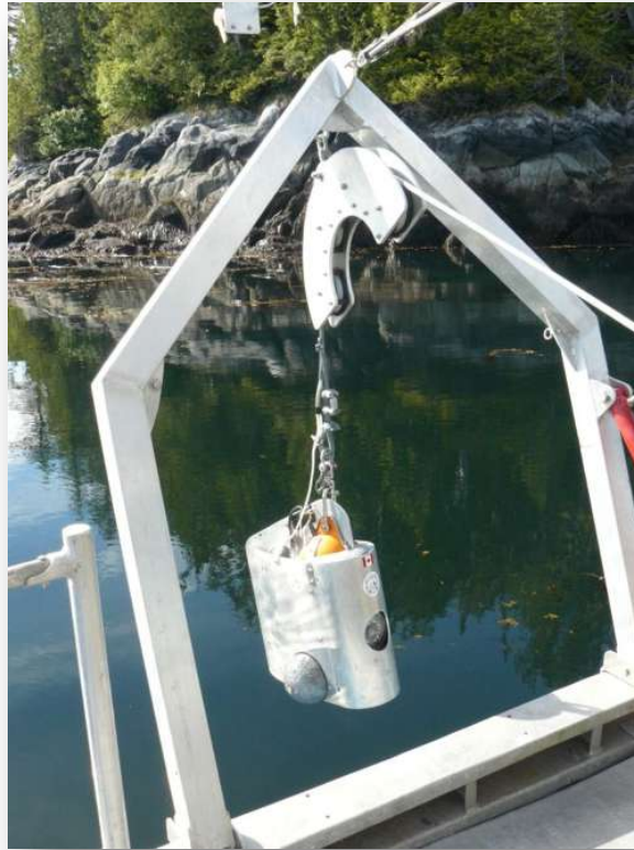
Figure 2. Towed video camera system about to be deployed.
